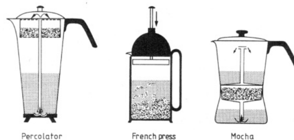
Figure 1. Brewing principles for percolated, French press (cafetiere or plunger), and mocha coffees.
